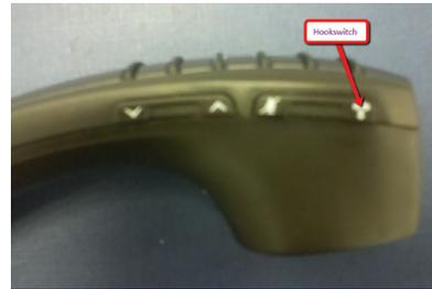
5. To pair the headset to the phone, perform step 3, then press and hold the silver, crescent-shaped hookswitch at the top of the headset until the blue LED on the headset blinks. The screen on the phone will prompt you if you want to pair this device. Press **“Yes”**. Press **“Close”**.
