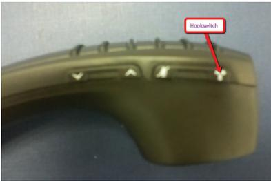
5. On the headset, the silver, crescent-shaped button is the hookswitch. The button on the top of the headset can be pressed down to mute and unmute the microphone or it can be slid forward or backward to increase/decrease volume. Operations of the controls on the headset will be reflected on your OfficeSuite® phone.
