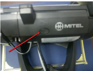
4. To pair the handset to the phone, perform step 3, then press and hold the hookswitch until the blue LED on the handset blinks. The screen on the phone will prompt you if you want to pair this device. Press **“Yes”**. Press **“Close”**.
