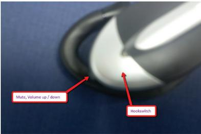
6. To receive an incoming call, press the hookswitch momentarily. Disconnect the call the same way. **NOTE: If engaged in a call and a second call comes in, pressing hookswitch will disconnect caller 1 and connect you to caller 2.**
