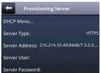
10. Change the entry in the **Server Address** field to **ps.broadviewnet.com** (you can use the keyboard icon in the top right corner to input, or use the number pad). Press **OK** when done, then press the **back** arrow until the **Network Configuration** screen appears.
